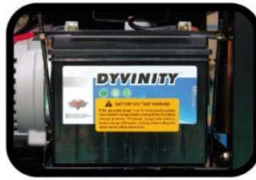
STEP 2. Connect the battery before starting.
